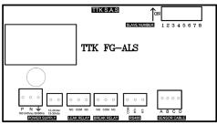
To connect the various cables (leader cable, power supply and relays) at the corresponding connector block.
